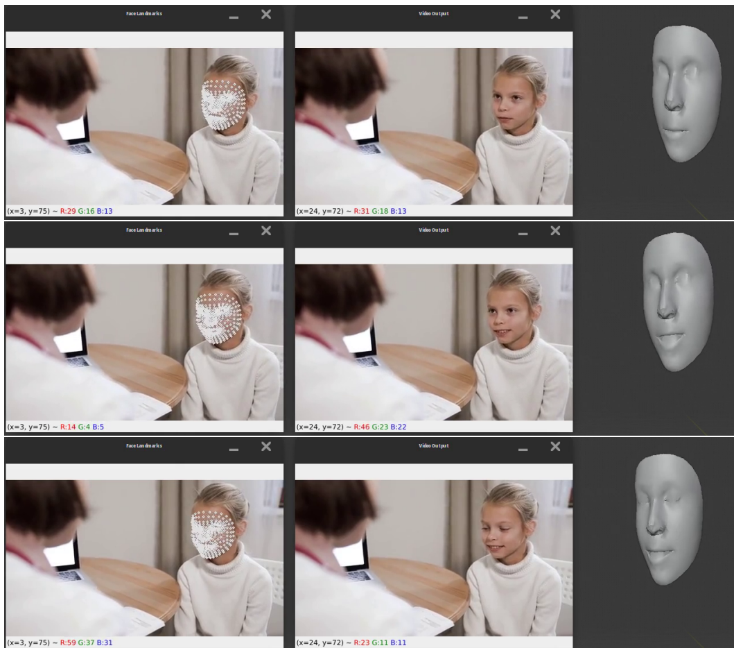
Figure 3.6: Facial landmark transfer from input video to 3D Face mesh.
