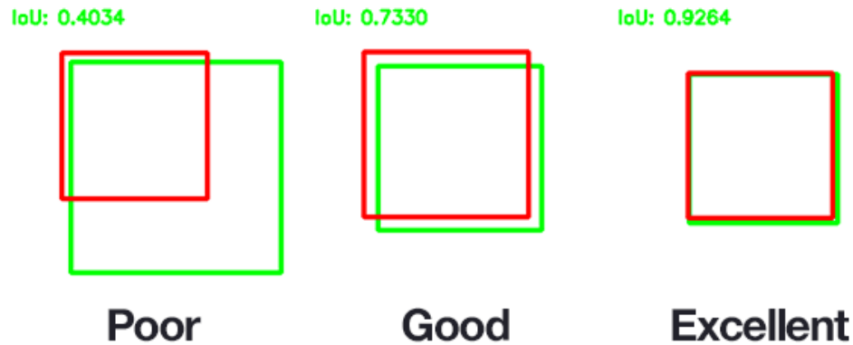
Figure 4.5: Example 3 of how Intersection over Union (IoU) yields different results based on the overlap of the prediction and the ground truth, illustrated by the use of bounding boxes. The values range from 0 to 1, where values around 0.4 indicates poor segmentation performance, values of 0.73 indicates good performance and values of 0.92 indicates excellent performance.
