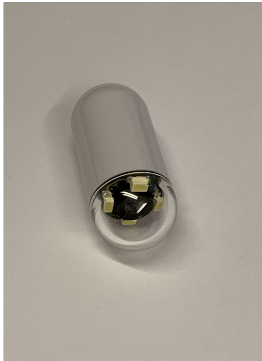
Figure 2.4: The image shows an Olympus EC-S10 endocapsule. Photo: Sigrun Losada Eskeland, Bærum Hospital.
