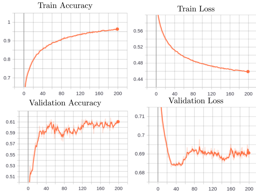
Figure 5.8: The figure shows train and validation accuracy and loss during training of ResNet50 pre-trained on ImageNet using the CLSF-DAT dataset combined with generated generated polyp videos. The dataset is unbalanced.
